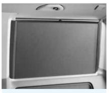
Roller sunblinds Sunblinds with a roller mechanism are fitted to the side windows of the rear passenger compartment. They help reduce build up of heat and shield occupants from dazzle.
